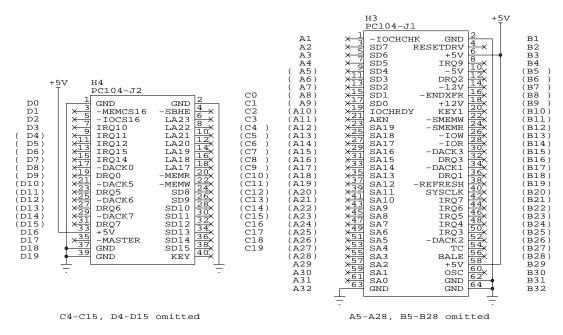
The FM430 implements a subset of the PC/104 specification in the form of two connectors that provide only +5V and GND for PC/104 modules. Only a total of 32 pins are implemented, 16 on J1 and 16 on J2. By adding up to 4 8-pin connectors to the FM430, PC/104 modules can be plugged directly into the FM430 to obtain +5V power and GND. No other connections between the PC/104 bus and the CubeSat Kit Bus are provided.
