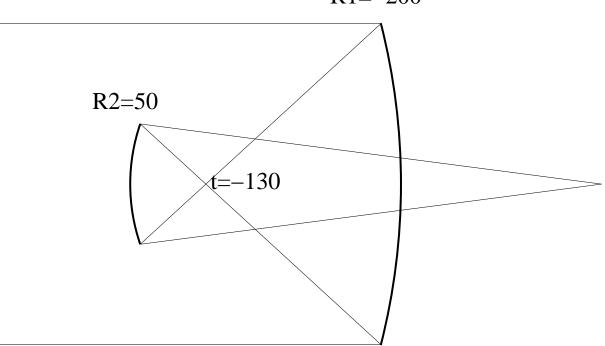
I will solve this problem by ending a ray through the system parallel to the optical axis, and use it's location and direction as it emerges to compute the focal length and focus location.
