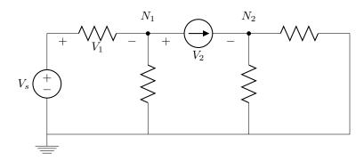
5. In the figure below, I = 8A. With a multimeter we measure (w.r.t. Gnd) 60V at  $N_2$ . Using nodal analysis and other techniques, find  $V_s$ ,  $V_1$ ,  $V_2$ , and the measurement we would expect to get at  $N_1$  (w.r.t. Gnd).
