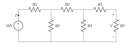
2. Given the figure below, find I and V using circuit reduction and other techniques.
