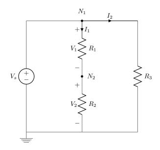
4. Given the figure below,  $V_s = 10$  V. With a multimeter we measure (w.r.t. Gnd) 4V at  $N_1$  and 7V at  $N_2$ . Find  $V_1$  and  $V_2$ .
