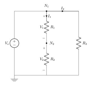
4. Given the figure below,  $V_s=10\mathrm{V}$ . With a multimeter we measure (w.r.t. Gnd) 4V at  $N_1$  and 7V at  $N_2$ . Find  $V_1$  and  $V_2$ .
