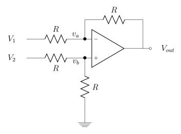
(a) Write an expression for  $V_{out}$  in terms of  $V_1$  and  $V_2$ . Show all your work and label important information on the circuit.
