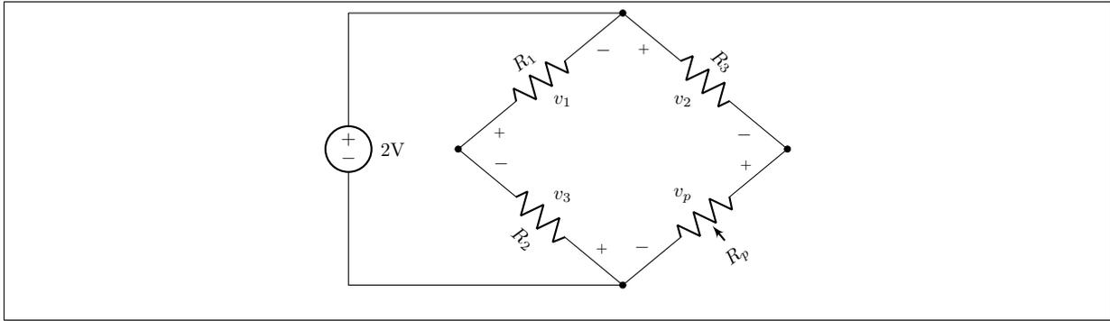
**Figure 3:** The Wheatstone bridge is a tool to sort resistors. It works using voltage division and standard ratios. When the ratio of  $R_1$  to  $R_2$  is the same as between  $R_3$  and  $R_p$ , then there will be no difference in voltages, and no current will flow between nodes. If  $R_1$  is  $10\text{ k}\Omega$  and  $R_2$  is  $50\text{ k}\Omega$ ,  $R_3$  and  $R_p$  would need to match a 2:1 ratio.
