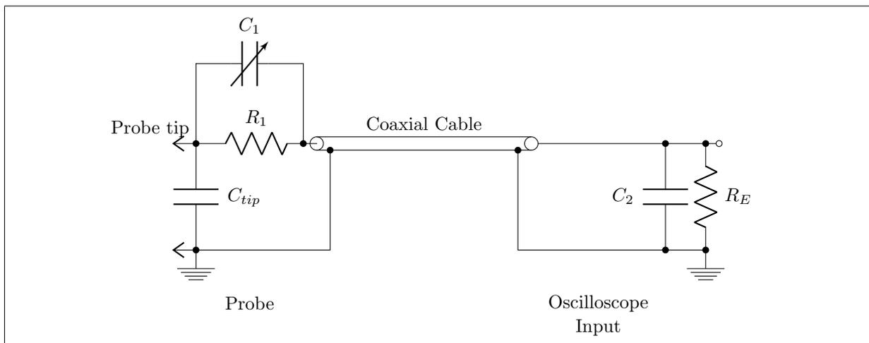
**Figure 1:** The internal circuitry of the Oscilloscope Probe. For a x1/x10 Probe  $R_1$  switches from a 1 M $\Omega$  to a 10 M $\Omega$  resistor.  $C_1$  changes when the probe is calibrated.
