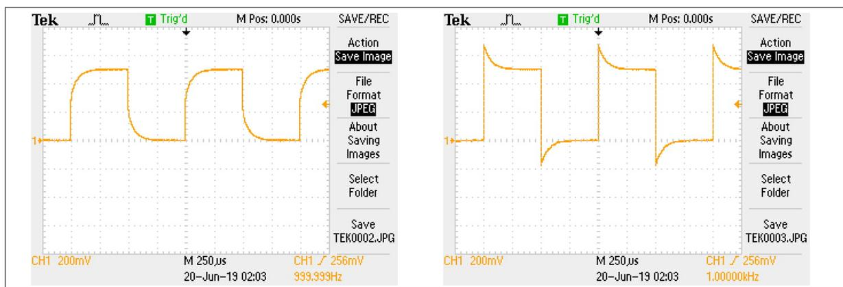
**Figure 2:** The figure on left side shows an example of a square wave measured through an over-damped probe, while the figure on right side shows the same waveform measured with an under-damped probe
