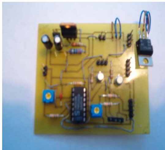
Figure 7: Aerial beacon control board.
