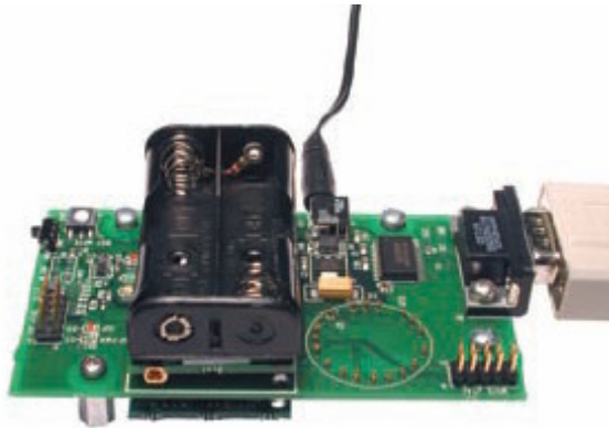
Figure 7: Base Station with micaZ and serial port connected, courtesy of ATmega
