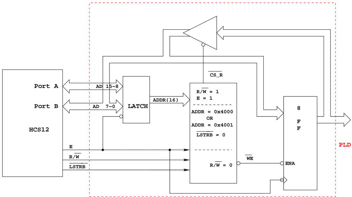
Writing to address 0x4001 (ADDR = 0x4000 or 0x4001, LSTRB low, R/W low) will bring WE low. On the high-to-low transition of E with WE low, the data into the flip-flops
