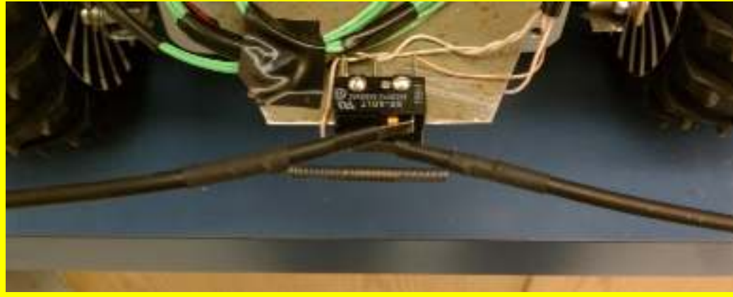
Figure 14 – Immediate Proximity Violation Detection Sensor
