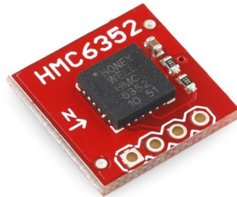
Figure 4.3.3: The Honeywell HMC6352 Compass
