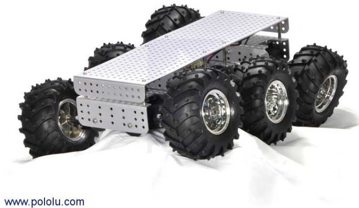
Figure 4.3.1: The Polulu Dagu Wild Thumper All Terrain Chassis [5]
