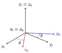
• e-frame rotated away from i-frame by angle  $\theta$  about  $z_i \equiv z_e$
