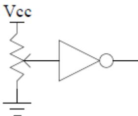
Figure 2. Changing the input to the inverter
