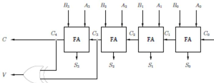
Figure 1: 4-bit Adder
