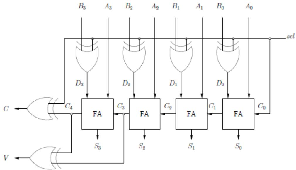
Figure 2: 4-bit Adder/Subtractor.
