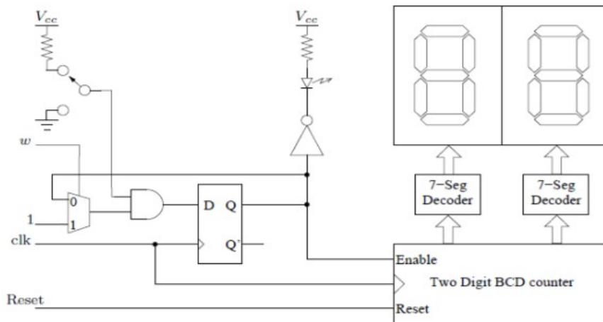
**Figure 1:** Circuit for Testing Your Reaction Speed
