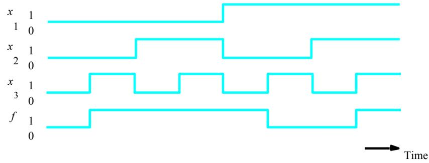
Fig. P2.4. A timing diagram representing a logic function.
