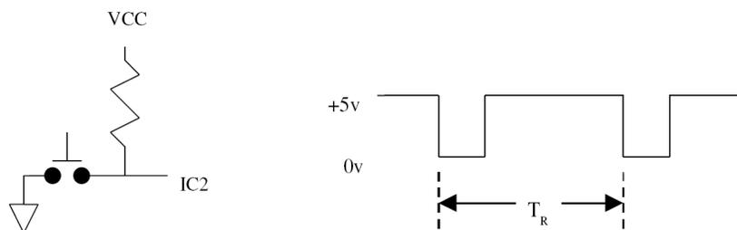
**Figure 1.** Circuit to measure speed of button pushing
