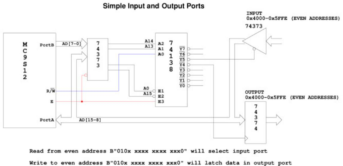
**Figure 1.** Block diagram of the HCS12 output port at address 0x4001
