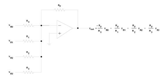
• By using input resistors which scale by factors of 2, a summing op amp can produce an output which follows a binary pattern
