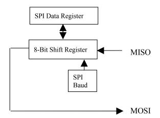
• To read data from the SPI, you read from the SPIDR after the transmission has completed.
