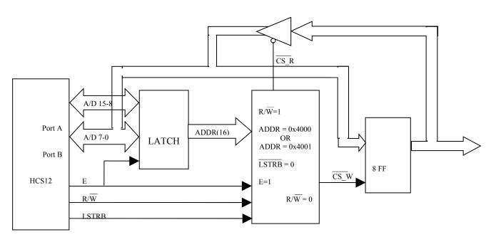
Writing to address 0x4001 will bring  $CS\_W$  low. On the high-to-low transition of E,  $CS\_W$  will go high, latching the data into the flip-flops
