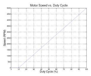
The motor doesn't start rotating until it is driven with a 10% duty cycle, after which it will increase speed linearly with the increase in duty cycle.
