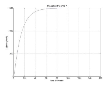
With this value of k, it will take about 1 minute for the motor to get to the desired speed.
