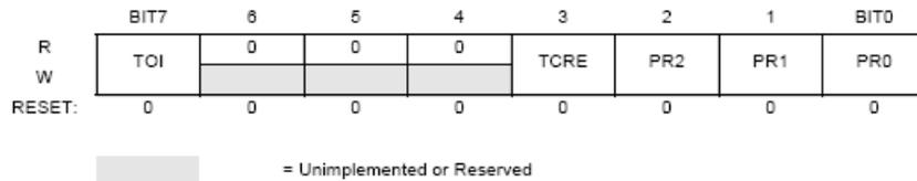
**Figure 3-11 Timer System Control Register 2 (TSCR2)**
