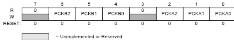
**Figure 3-4 PWM Prescale Clock Select Register (PWMPRCLK)**
