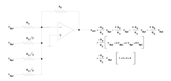
• By using switches on the input resistors, a summing op amp can produce an output which is a binary number (representing which switches are closed) times a reference voltage
