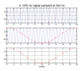
• A 1,050 Hz signal sampled at 500 Hz looks like a 50 Hz signal
