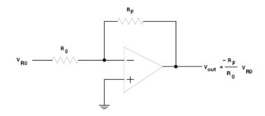
• An inverting op amp can produce an output voltage which is a linear combination of several input voltages
