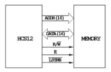
WRITE: a) HCS12 puts address on address bus and puts data on data bus
