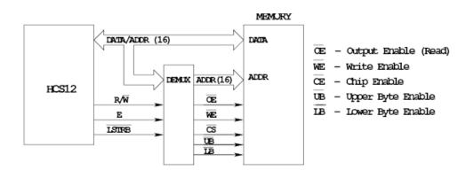
HCS12 has 16-bit address and 16-bit data buses Requires 35 bits Not enough pins on HC12 to allocate 35 pins for buses and pins for all other functions
