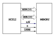
READ: a) HCS12 puts address on address bus
