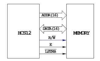
HCS12 has 16-bit address and 16-bit data buses Requires 35 bits Not enough pins on HCS12 to allocate 35 pins for buses and pins for all other functions
