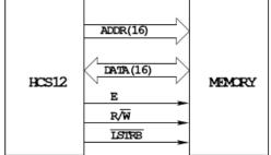
HCS12 has 16 bit address bus – can access 65536 bytes 1024 bytes = 1 kB 65536 bytes = 64 kB
