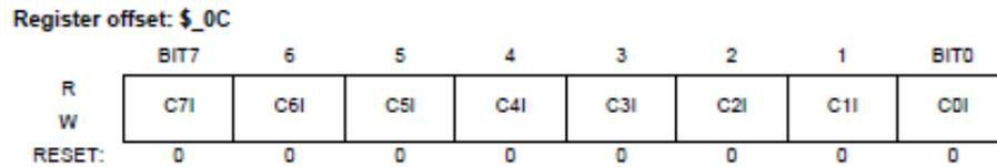
Figure 3-10 Timer Interrupt Enable Register (TIE)
