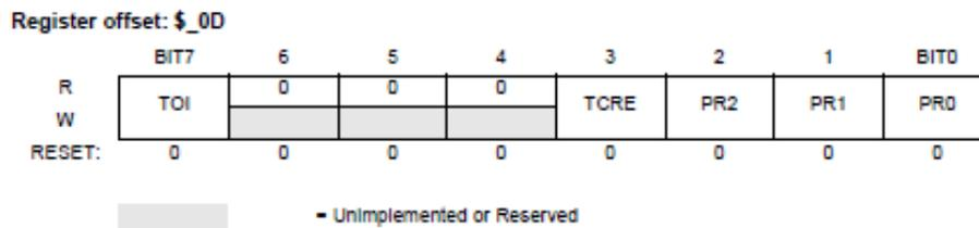
Figure 3-11 Timer System Control Register 2 (TSCR2)
