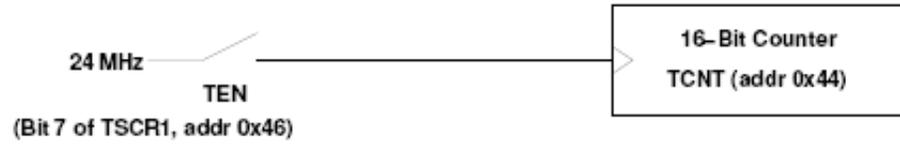
To enable timer on MC9S12, set Bit 7 of register TCSR1:
