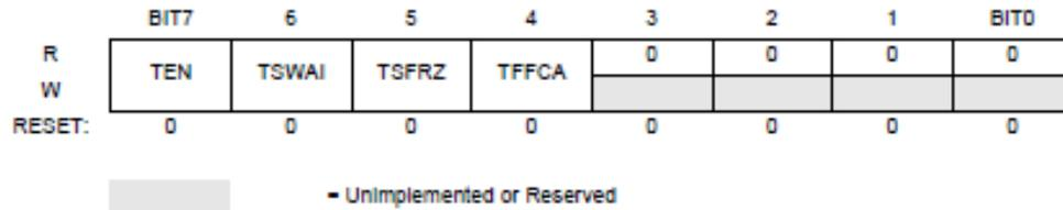
Figure 3-6 Timer System Control Register 1 (TSCR1)
