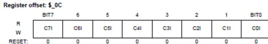
Figure 3-10 Timer Interrupt Enable Register (TIE)
