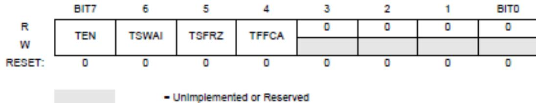
Figure 3-6 Timer System Control Register 1 (TSCR1)
