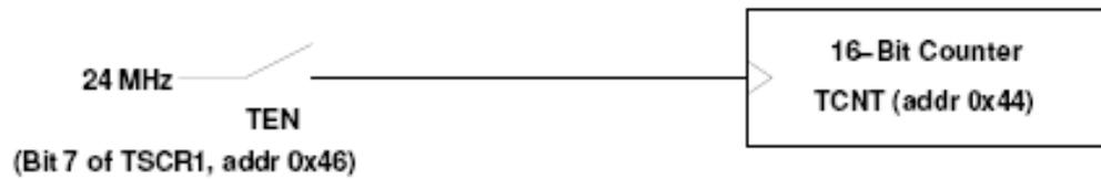
To enable timer on MC9S12, set Bit 7 of register TCSR1:
