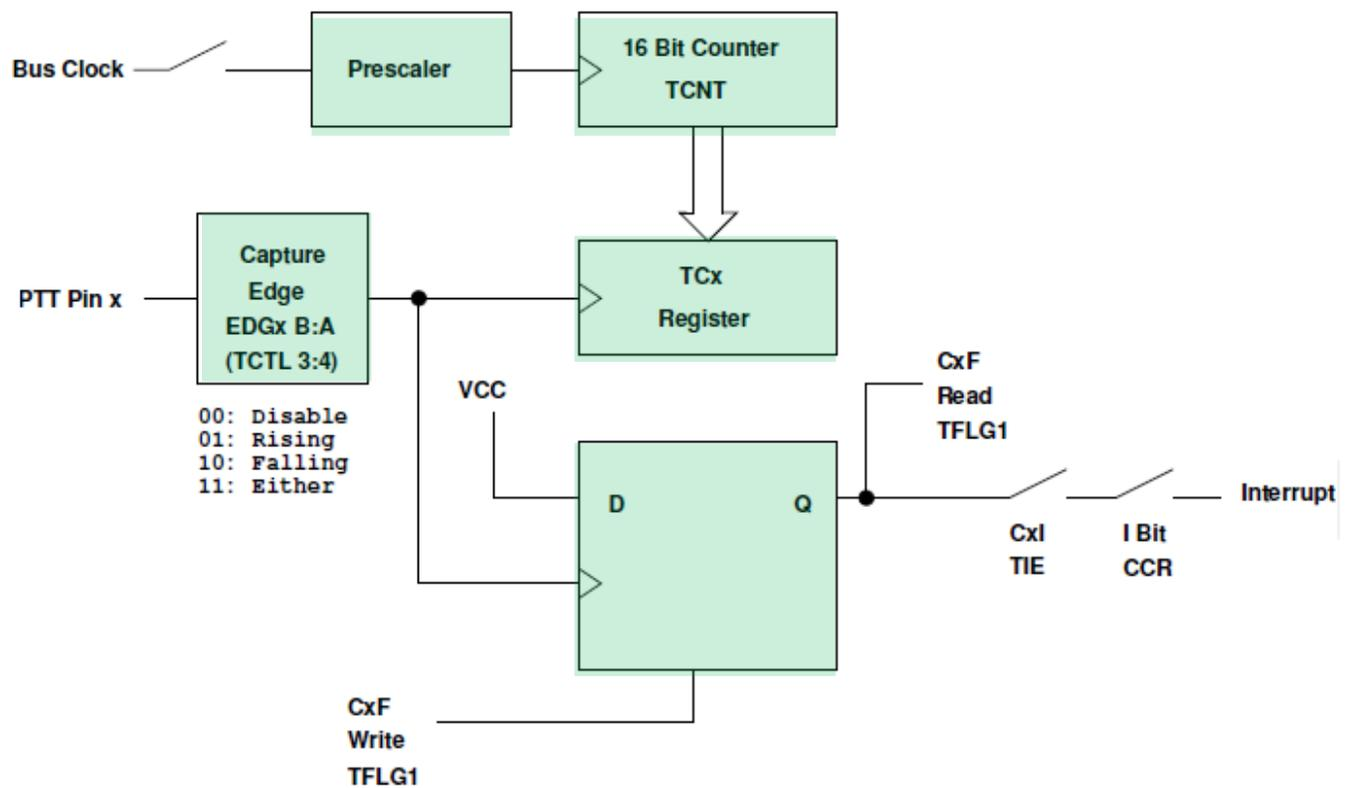
**Registers used to enable Input Capture Function**
