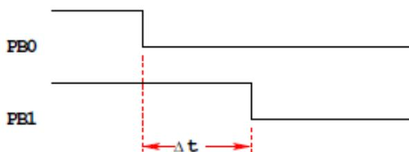
**Solution:** Latch TCNT on falling edge of signal
