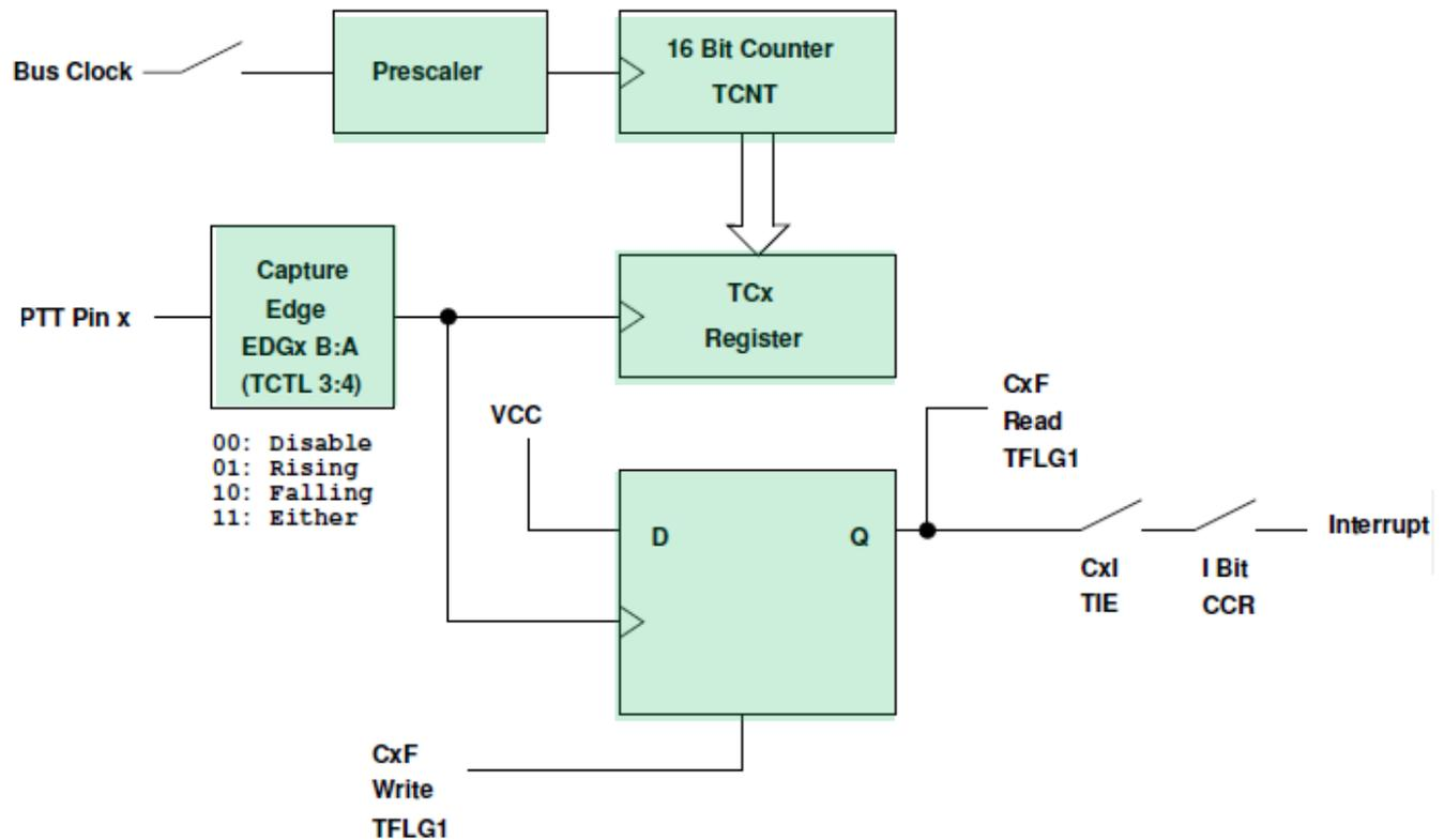
Write a 0 to the bits of TIOS to make those pins input capture
