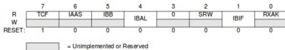
Figure 3-5 IIC Bus Status Register (IBSR)
