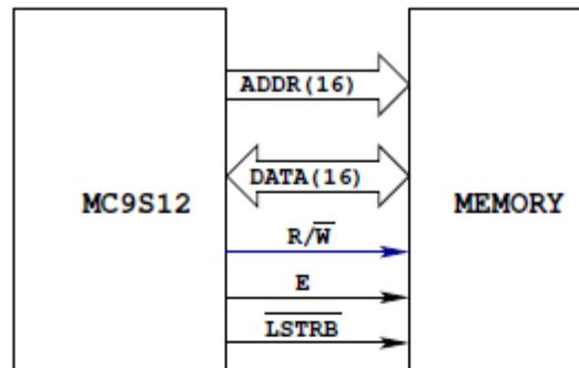
**READ:** MC9S12 puts address on address bus
