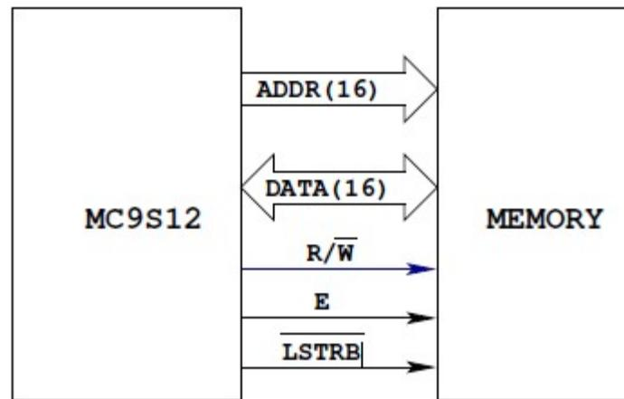
MC9S12 has 16-bit address and 16-bit data buses
