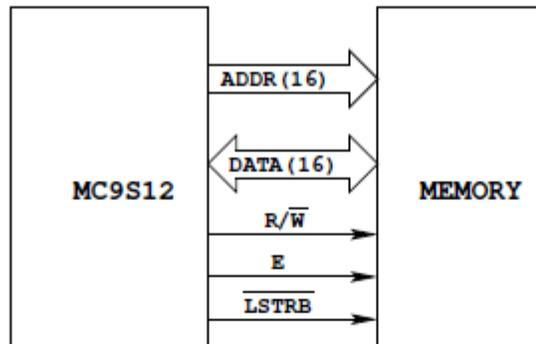
**WRITE:** MC9S12 puts address on address bus
