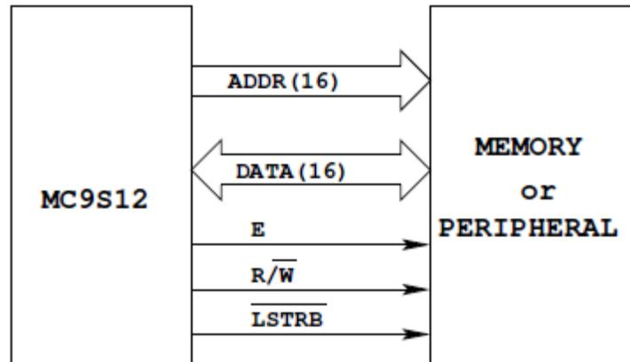
MC9S12 has 16 bit address bus – can access 65536 bytes
