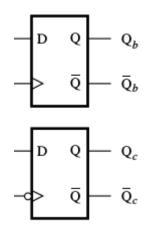
In the symbols we use the > mark to denote that the flip-flop responds to the active edge of a **clock signal**.
