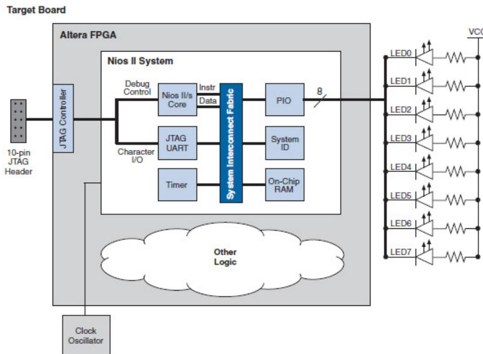
**Figure 1.** Block diagram of the embedded system (taken from Nios II Hardware Development Tutorial).
