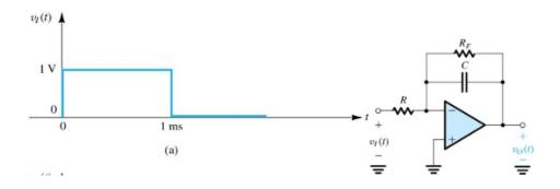
4.- (Exa 2.8) The op amp below, is specified to have output saturation voltages of  $\pm 13$  V and output current limit of  $\pm 20$  mA.
