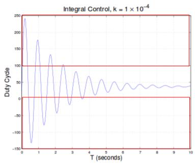
• To get this oscillating response, the duty cycle must go over 100%, and below 0%, which is clearly impossible.
