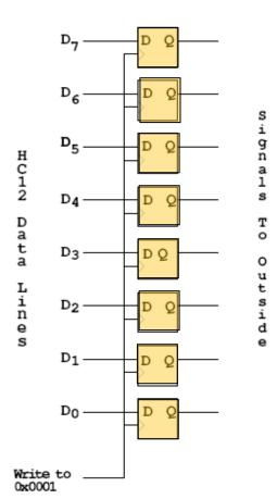
Any write to address \$01 latches data into FF, so data goes to external pins
