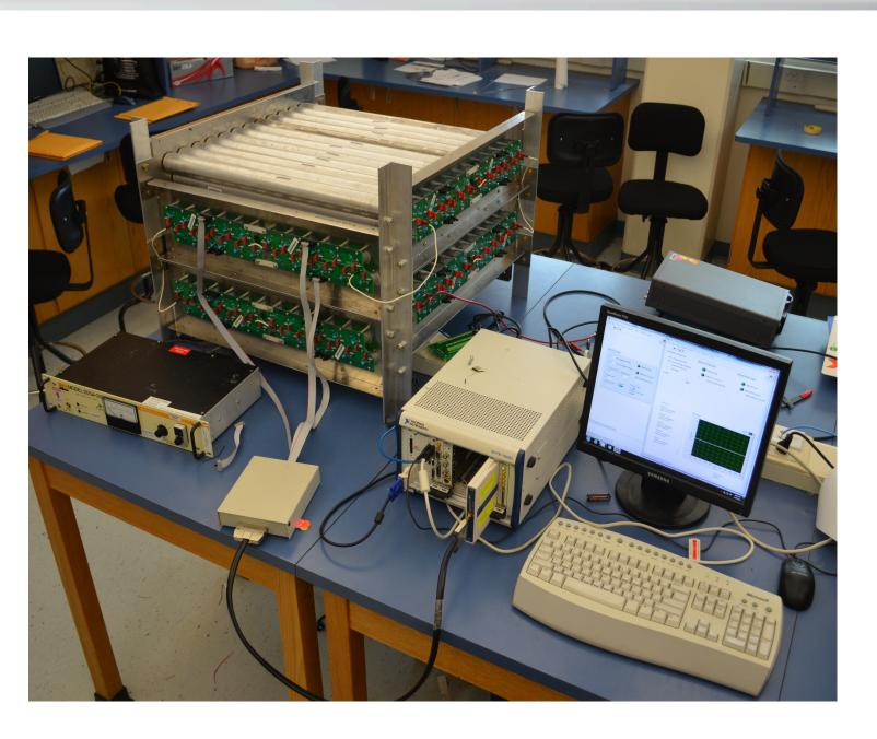
Figure 5. Muon Tracker and Acquisition Hardware
