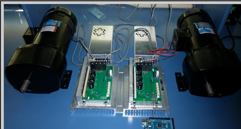
Figure 4. Motor, Power Supply, and Driver Configuration
