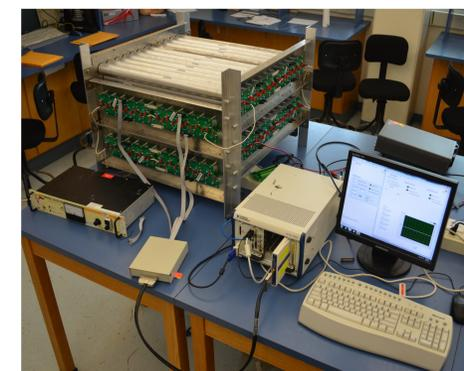
Figure 5. Muon Tracker and Acquisition Hardware
