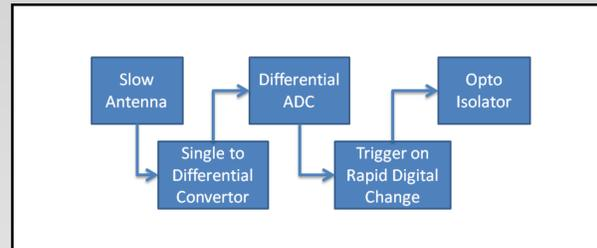
Figure 3. Digital Consecutive Voltage Differential Detector Block Diagram
