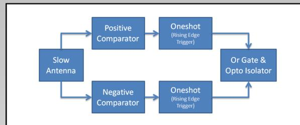
Figure 2. Analog Threshold Detector Block Diagram
