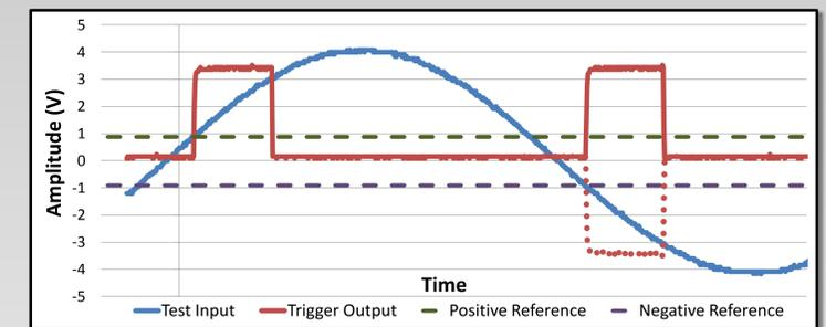
Figure 6. Positive Pulse Generation at Threshold Crossing
