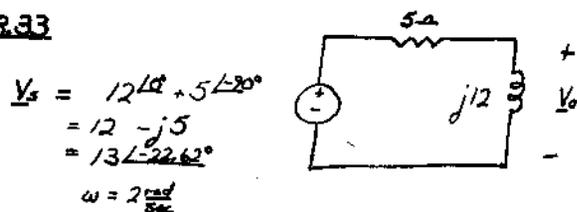
$$a) \underline{V}_o = \frac{(13\angle -22.62^\circ)(j12)}{5+j12} = \frac{(12-j5)(j12)}{5+j12} = 12 \Rightarrow \underline{V}_o(t) = 12\cos 2t \text{ V}$$
