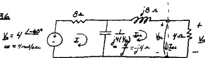
\*  $V_{oc}$ :  $V_{oc} = \frac{(4\angle-40^\circ)(-j4)}{8-j4} = \frac{4\angle-40^\circ \cdot 4\angle90^\circ}{8.944\angle-26.57^\circ} = 1.79\angle-123.4^\circ = \frac{4}{\sqrt{5}}\angle-123.4^\circ$
