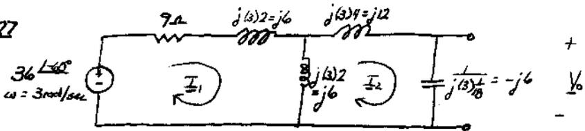
$$a) \text{ e } \underline{I}_1: -36 \angle 60^\circ + 9 \underline{I}_1 + j6 \underline{I}_1 + j6(\underline{I}_1 - \underline{I}_2) = 0$$
