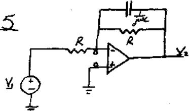
$$\begin{aligned} e^{i\omega t}: \frac{V - V_1}{R} + \frac{V - V_2}{jwC} + \frac{V - V_2}{R} &= 0 \\ \Rightarrow -V_1 - jwCRV_2 - V_2 &= 0 \\ \Rightarrow V_2(1 + jwCR) &= -V_1 \\ \Rightarrow H(j\omega) = \frac{V_2}{V_1} &= \frac{-1}{1 + jwCR} \end{aligned}$$
