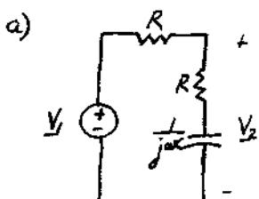
$$V_2 = \frac{V_1(R + \frac{1}{j\omega C})}{R + R + \frac{1}{j\omega C}} = \frac{V_1(j\omega CR + 1)}{j\omega C2R + 1} \Rightarrow H(j\omega) = \frac{1 + j\omega CR}{1 + j\omega C2R}$$
