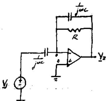
$$e^{i\omega t}: \frac{V - V_1}{jwC} + \frac{V - V_2}{jwC} + \frac{V - V_2}{R} = 0$$
