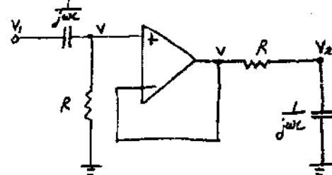
$$e^{+i\omega t}: \frac{V - V_1}{j\omega C} + \frac{V - 0}{R} = 0$$
