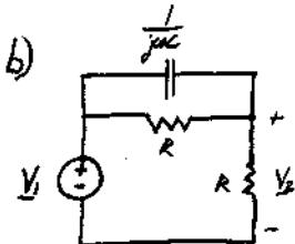
$$V_2 = \frac{V_1 R}{\left( R + \frac{1}{j\omega C} \right) + R} = \frac{V_1 R}{R + R + \frac{1}{j\omega C}} = \frac{V_1 R}{R + \frac{1}{j\omega CR + 1}}$$
