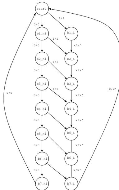
You could also implement this with just three states and a 3-bit counter. Have the counter keep track of the number of bits. When the number of bits is seven, go back to the START state:
