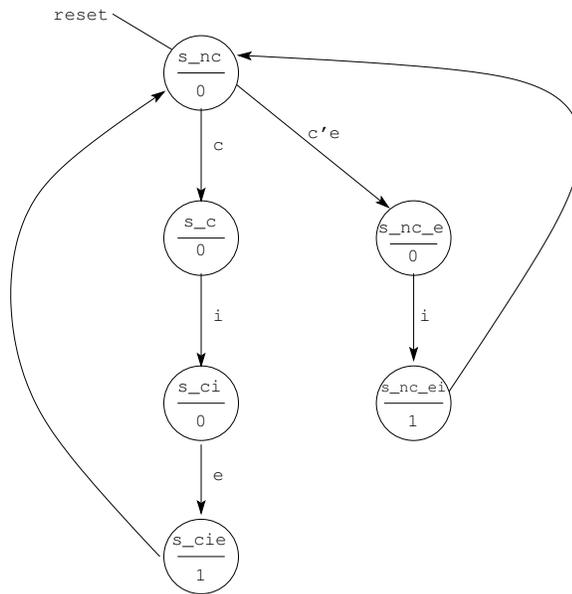
The above state diagram shows only one path to get to the state  $s_c$  (the state where the last letter was c). However, if you are in any of the other states (e.g., state  $s_{nc_e}$ ) and a  $c$  comes along, you need to go the state  $s_c$ . Similarly, if you are in any state except  $s_c$  and an  $e$  comes along, you need to go to the state  $s_{nc_e}$ . This gives a lot more paths to get to the states  $s_c$  and  $s_{nc_e}$ :
