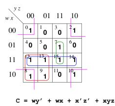
Each output function of the PAL only has three input OR gates, but C needs four terms to be ORed together. Write C = D + xyz, where D = wy' + wx + x'z', and feed D back into PAL array to generate C.
