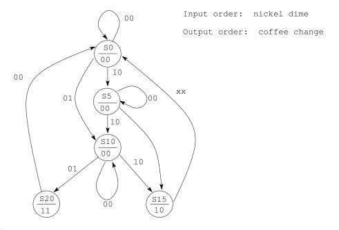
I assume that another coin cannot be inserted betwen states S15 and S0, or between states S20 and S0. This is a reasonable assumption – it will take at least several milliseconds before a person can deposit another coin and the coin can fall into the coin box, while the time between state S15 and S0 is one clock cycle, probably less than a microsecond. (b) Assign states, and draw a state transition table.
