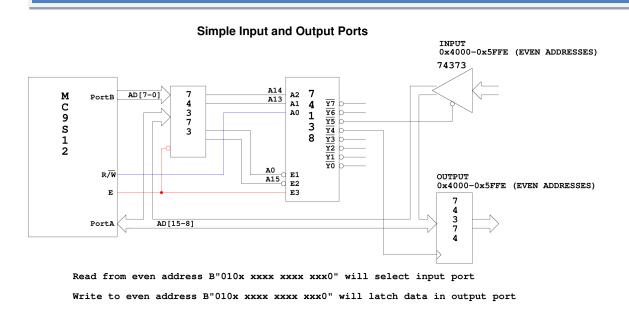
Figure 1: Block diagram of HCS12 output port at address 0x4001
