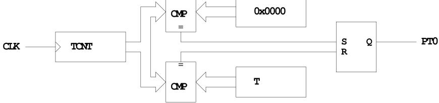
When TCNT = 0x0000, the output goes high When TCNT = T, the output goes low
