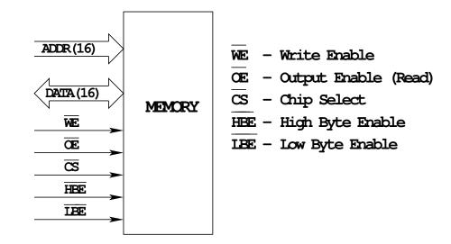
Memory needs separate address and data busses Need way to separate address and data • To talk to memory chip we will need to build a demultiplexer between the MC9S12 and the memory chip
